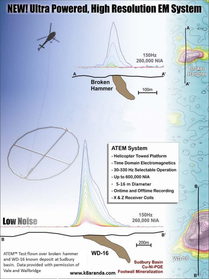
ATEM<sup>®</sup> a new helicopter towed, rigid platform, Time Domain EM System developed by Wally Boyko, designer of the first commercial Helicopter Time Domain System in 1999.
